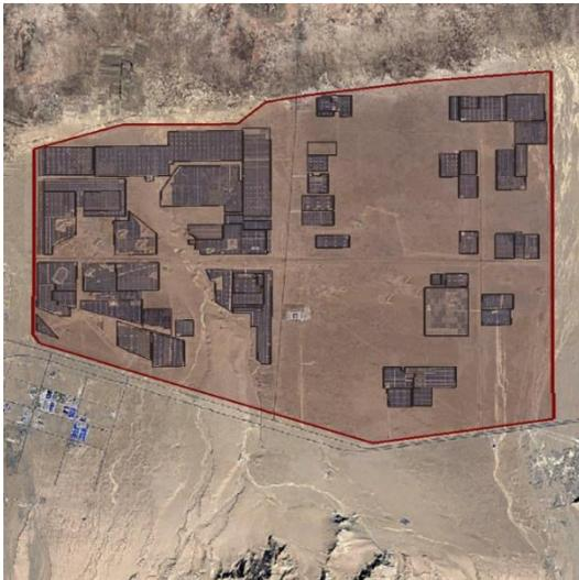
Located in the desert to the East of Golmud in Qinghai Province in China [this park](#) accommodates at least 55 solar power plants with a combined capacity of over 1,800 MW<sub>AC</sub>. It includes a 200 MW<sub>P</sub> plant by Huanghe – the largest individual solar power plant in the world, when it was first built in 2011.
